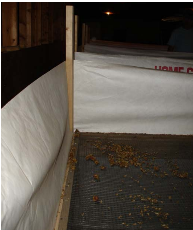
Inside of a home made oast, note the mesh screen installed partway up to allow air to circulate below and above the hops. Note the series of oasts in the background, enabling more volume to be drying simultaneously. Picture of Gene L'Etoile's Four Star Farms, MA. Photo credit r.wilson
