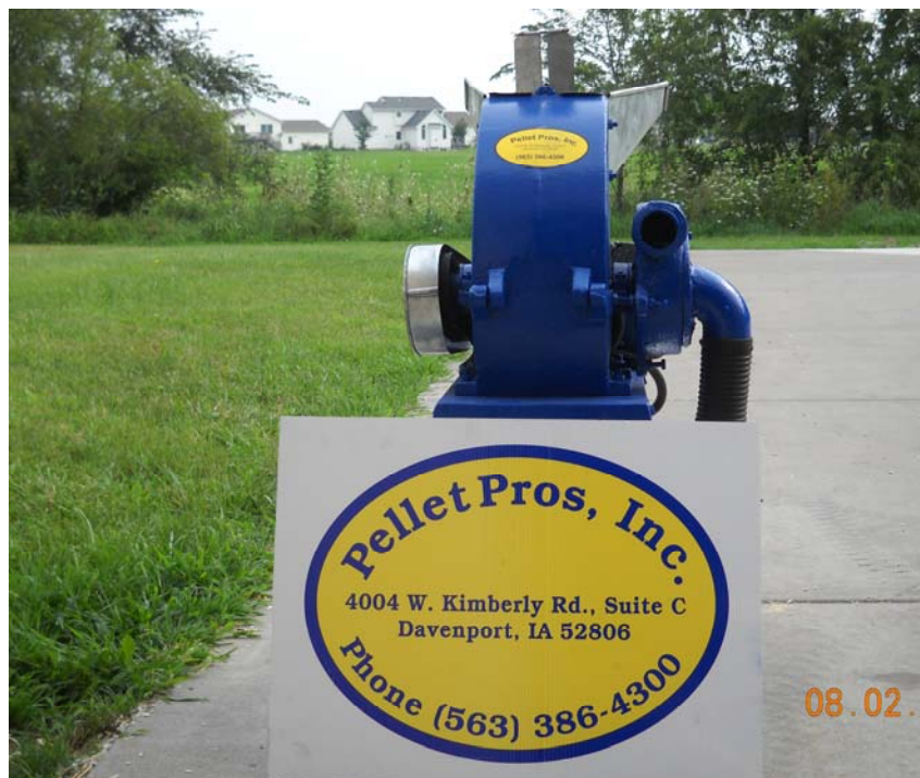
Small Scale Pellet Pros Hammermill. 130lb/hr capacity
