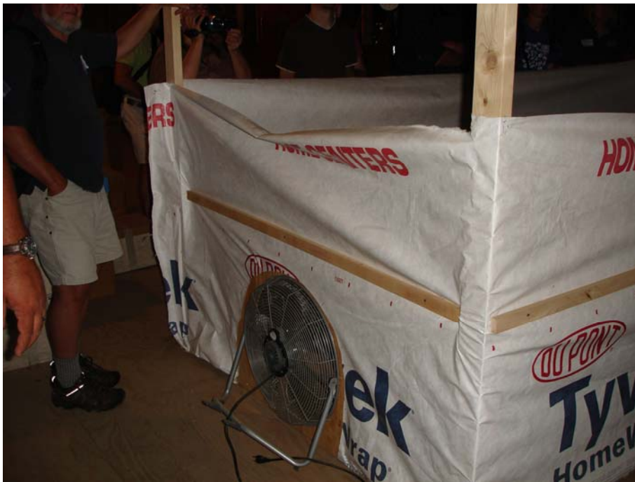
Exterior view of a home made oast. Supplies are simple 2x4's to create the frame, 1x2's to affix the screen, a 4'x8' screen, tyvek to form the walls, and a circular fan. Picture of Gene L'Etoile's Four Star Farms, MA. Photo credit r.wilson
